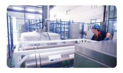
The company has a full set of cryogenic valve test equipment, including full-size liquid nitrogen pool, valve seat leakage flow meter, torque and test machine, helium detector, to provide capability and product research and development and production test.
